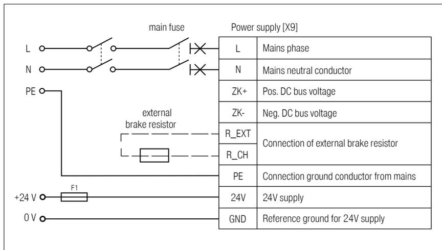
Figure 20: Connection of a BL 1-04 /C to the power supply [X9]
