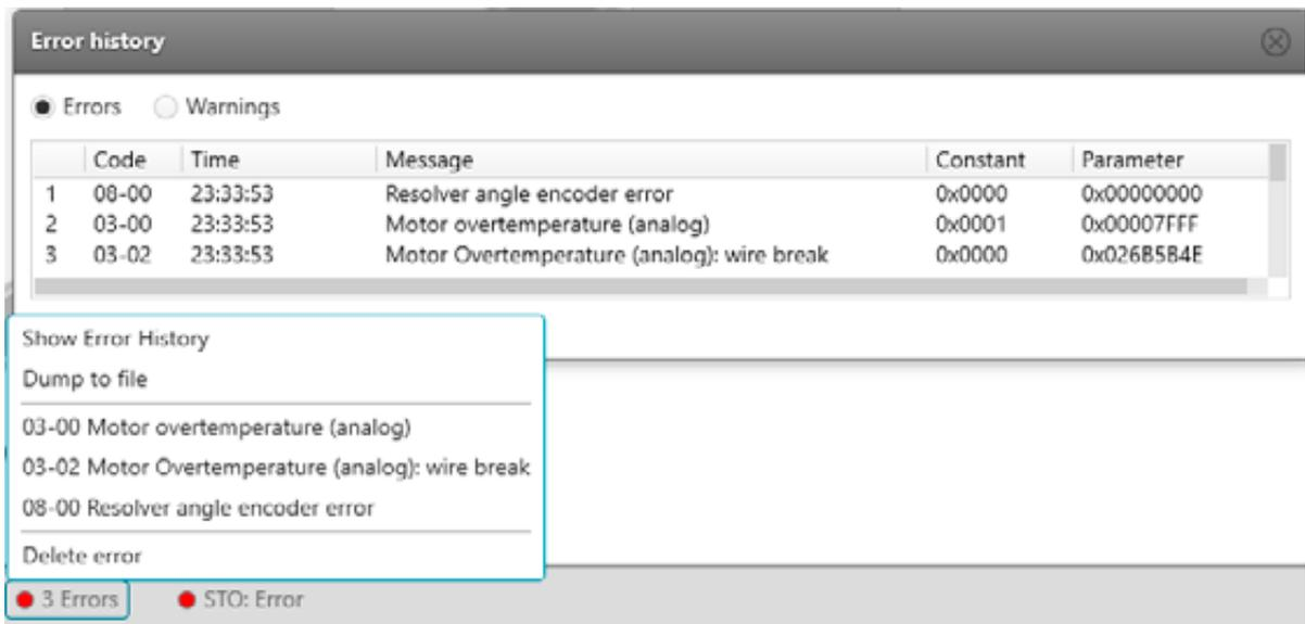
Figure 13: "Error buffer" and "Error messages" windows
