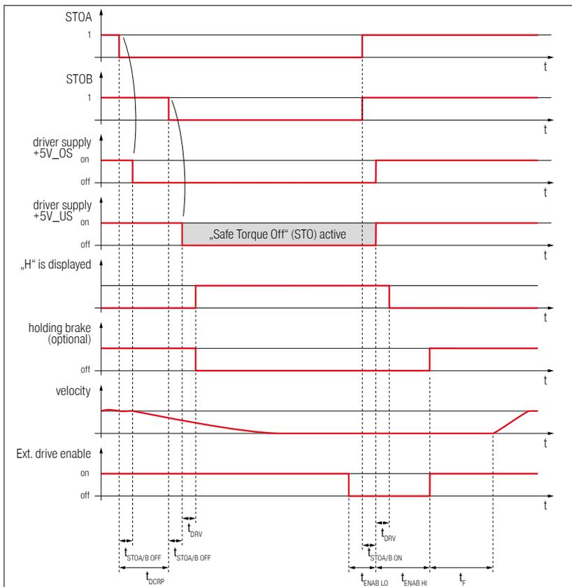
Figure 18: Time response of the activation of the STO safety function with a restart
