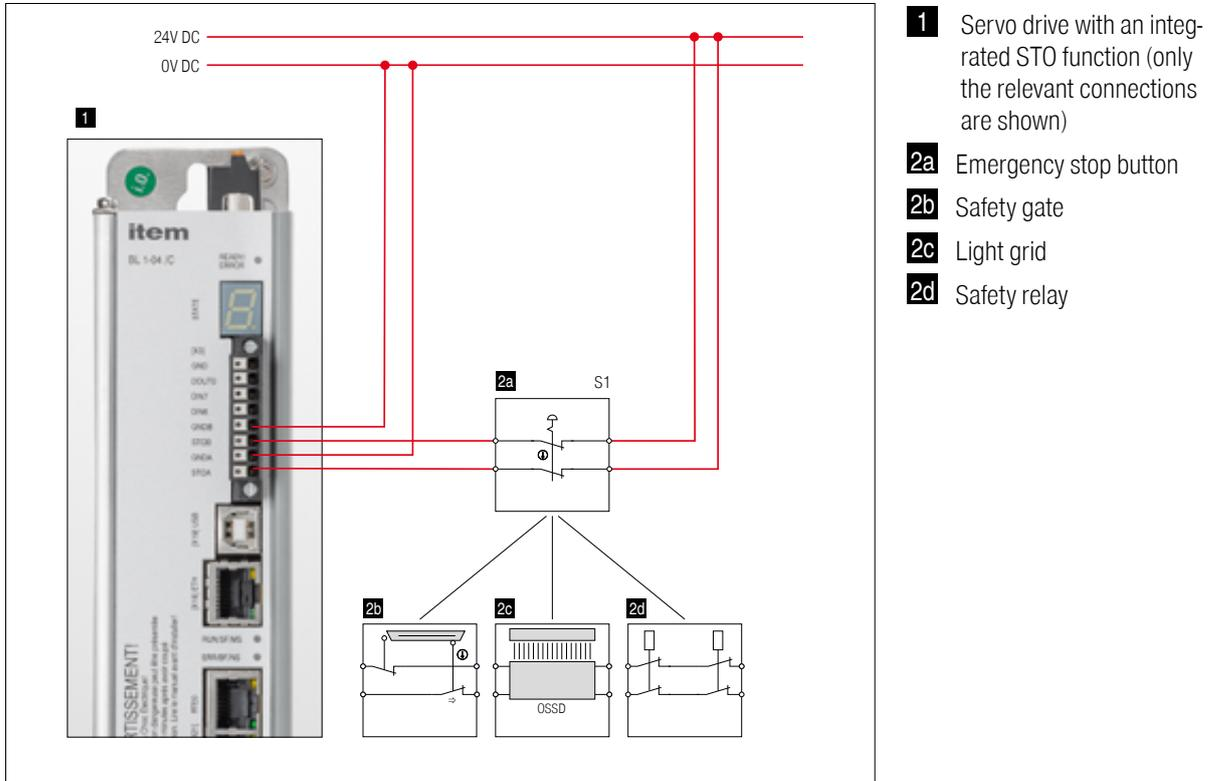
Figure 6: Connection of the integrated STO function (single-phase servo drive)
