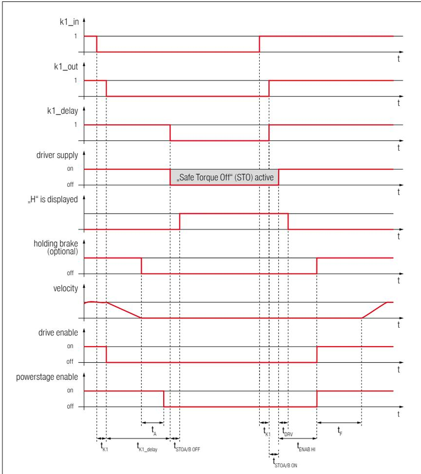
Figure 19: Time response during the activation of the SS1 safety function (external switching) with a restart
