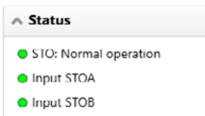
Figure 11: Safety module Status window
