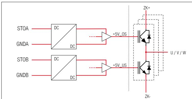
Figure 4: "Safe Torque Off" - principle of operation
