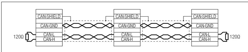
Figure 31: CAN bus cabling example
