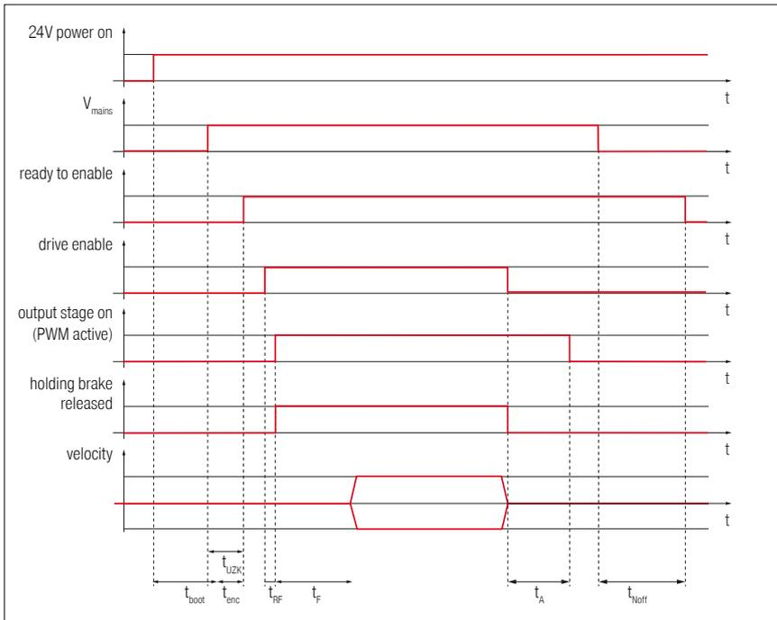
Figure 17: Time diagram of the servo drive
